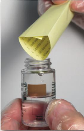
2. Add 5 drops of Solution 2 to the bottle of Solution 1 containing the sample, close and shake.
